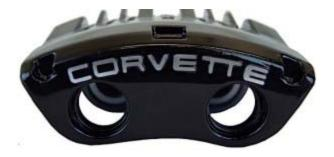
He continued, "The black brake calipers presented some challenges as well. The stock calipers were a real eyesore with the black wheels, and we couldn't just leave them. Again, the casting was inexpensive which created a lot of issues when it came to painting. The provider agreed to used a different metal which ultimately resulted in a caliper that was much stronger and heat resistant. These calipers were also used on the Camaro and Firebird in 1997."
