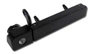
"The door handles are built with a very inexpensive metal, that get coated with a crinkle coat black finish to hide any imperfections. The metal is porous and not smooth enough to paint the body color," Heinricy said. "There were a few sets of handles completed successfully using body-filler to smooth the surfaces, but it took too long to complete, and that concept was scratched. One car did leave the plant with the blue door handles, which was a convertible; it was Tom Daleworth's car."
